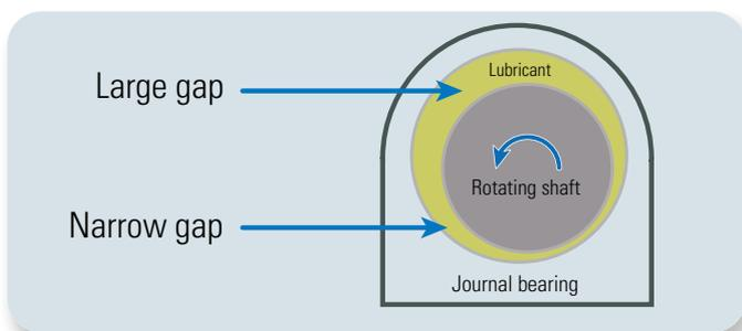
Figure 3. Converging gap of a journal bearing.
