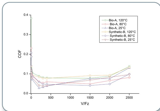
Figure 4. Stribeck curves generated under different temperatures.
