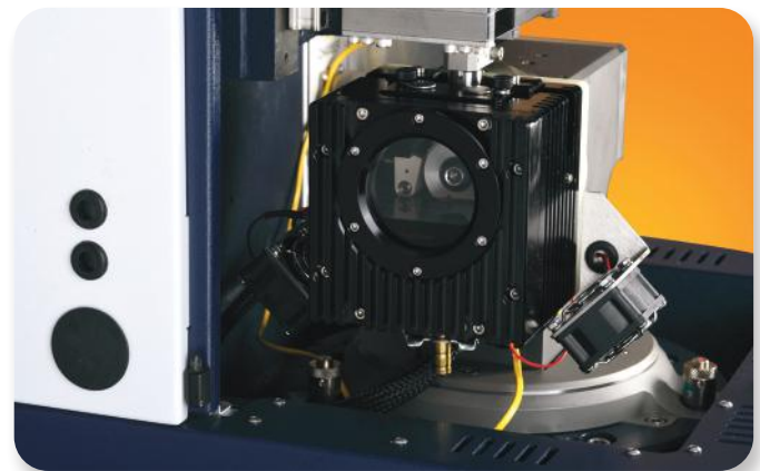
Figure 1. UMT TriboLab Liquid Heating Chamber on Block-On-Ring Module.
